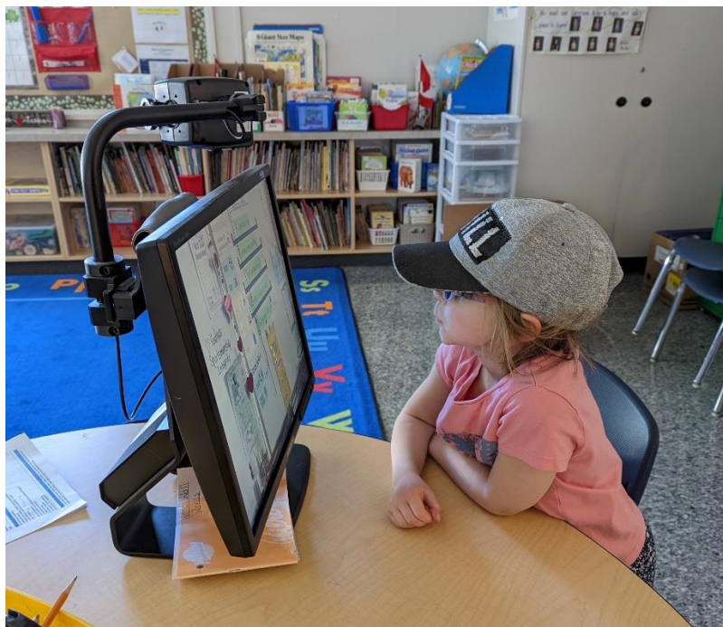
Closed Circuit Television (CCTV) - Video Magnifier used for enlarging images
